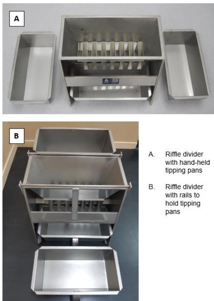
Figure 9: Riffle Divider and Tipping Pans
