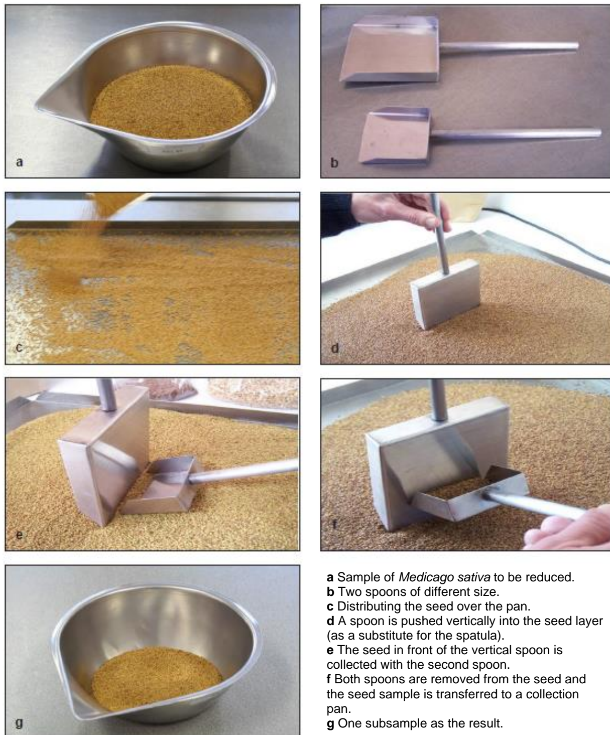
Figure 10: Sample reduction using the spoon method
