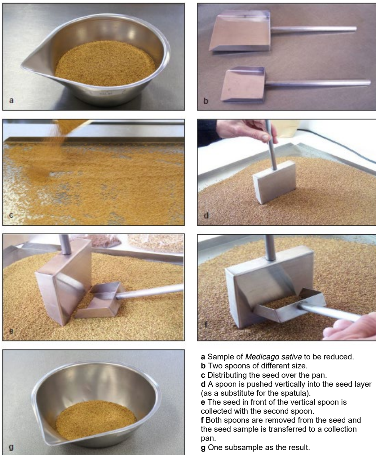
Figure 10: Sample reduction using the spoon method
